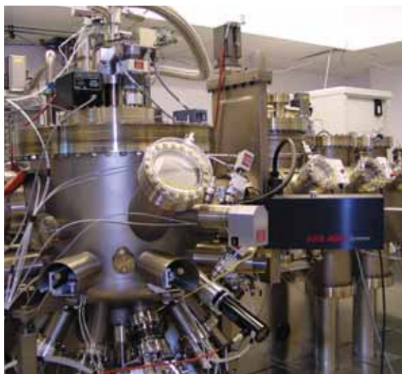
Reaktor MBE (Molecular Beam Epitaxy) w laboratorium (Top-GaN)
